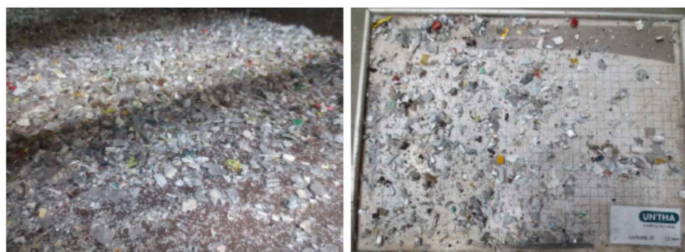
Figure 9. Shredding output of 12 mm in Company B shredding machine.
