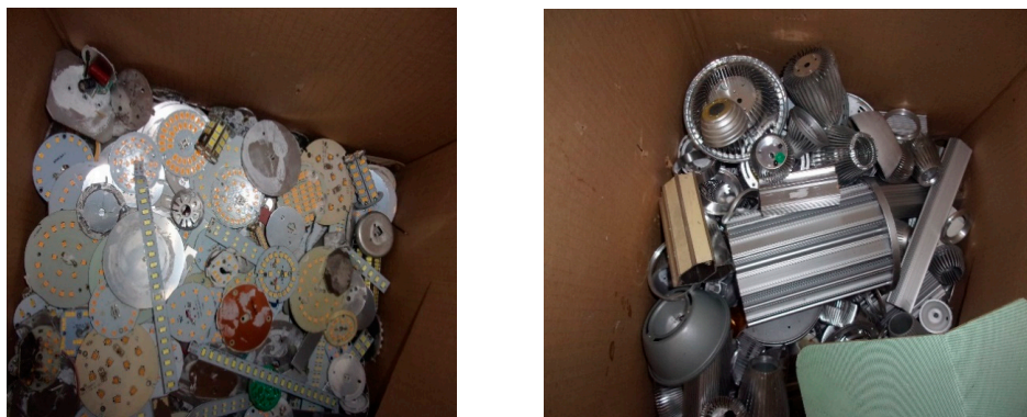
Figure 5. LED chip package and aluminum fraction of manual disassembly.
